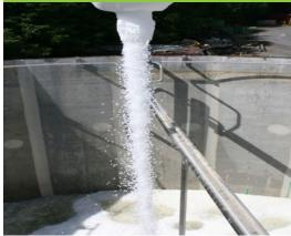
Bioreactor being filled with media.
